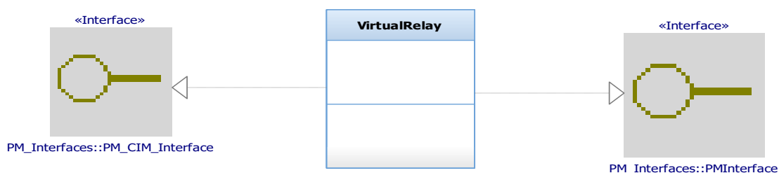
Figure 7.12: The software adapter linking the interfaces required by the CIT and the PIM.
